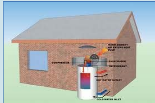
Heat Pump Hot Water System
